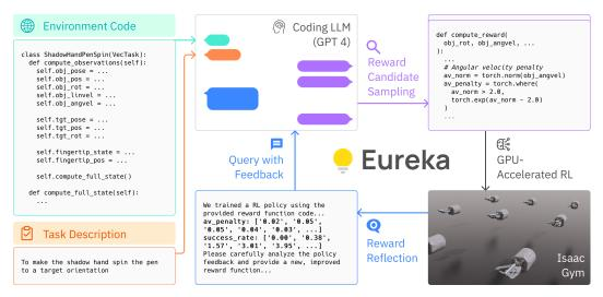
Figure 2: EUREKA takes unmodified environment source code and language task description as context to zero-shot generate executable reward functions from a coding LLM. Then, it iterates between reward sampling, GPU-accelerated reward evaluation, and reward reflection to progressively improve its reward outputs.
